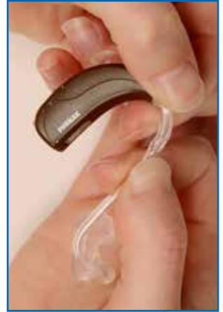
To wash the earmould you need to remove it from the hearing aid. To do this hold onto the tubing with one hand and the hearing aid in the other and ease the two bits apart, as shown. You may need to pull it fairly hard but this should not harm the hearing aid.
